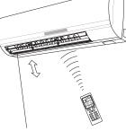
Flap of upward / downward position.
